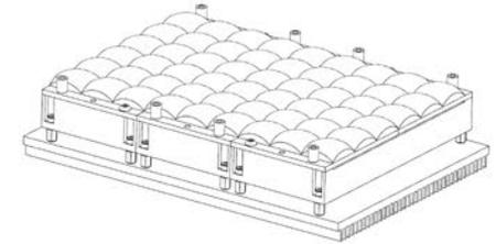
2 Place the attached round spacers in the holes of the removed wood screws.
