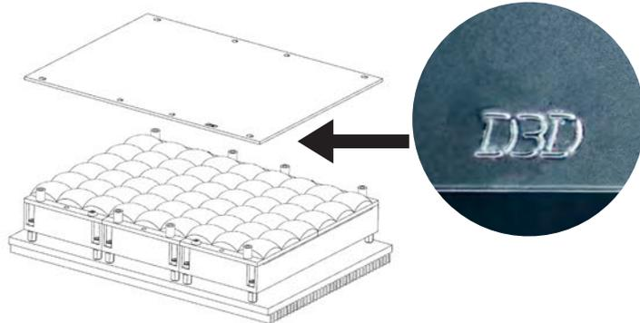
3 Remove the protective sticker on both sides of the diffuser and place it on the spacer so that the letters on the D3D are properly visible and the frosted side is up.
