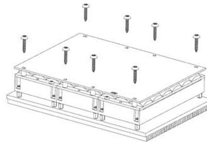
4 Secure the spacers and diffuser at the same time with the included wood screws.
