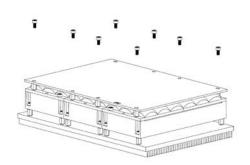
Fix the diffuser with the bolts removed in #1.
