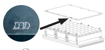
Remove the protective sticker on both sides of the diffuser and place it on the spacer so that the letters on the D3D are properly visible and the frosted side is up.
