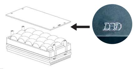
Remove the protective sticker on both sides of the diffuser and place it on the spacer so that the letters on the D3D are properly visible and the frosted side is up.
