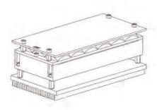
Remove the protective sticker on both sides of the diffuser and place it on the spacer so that the letters on the D3D are properly visible and the frosted side is up.
